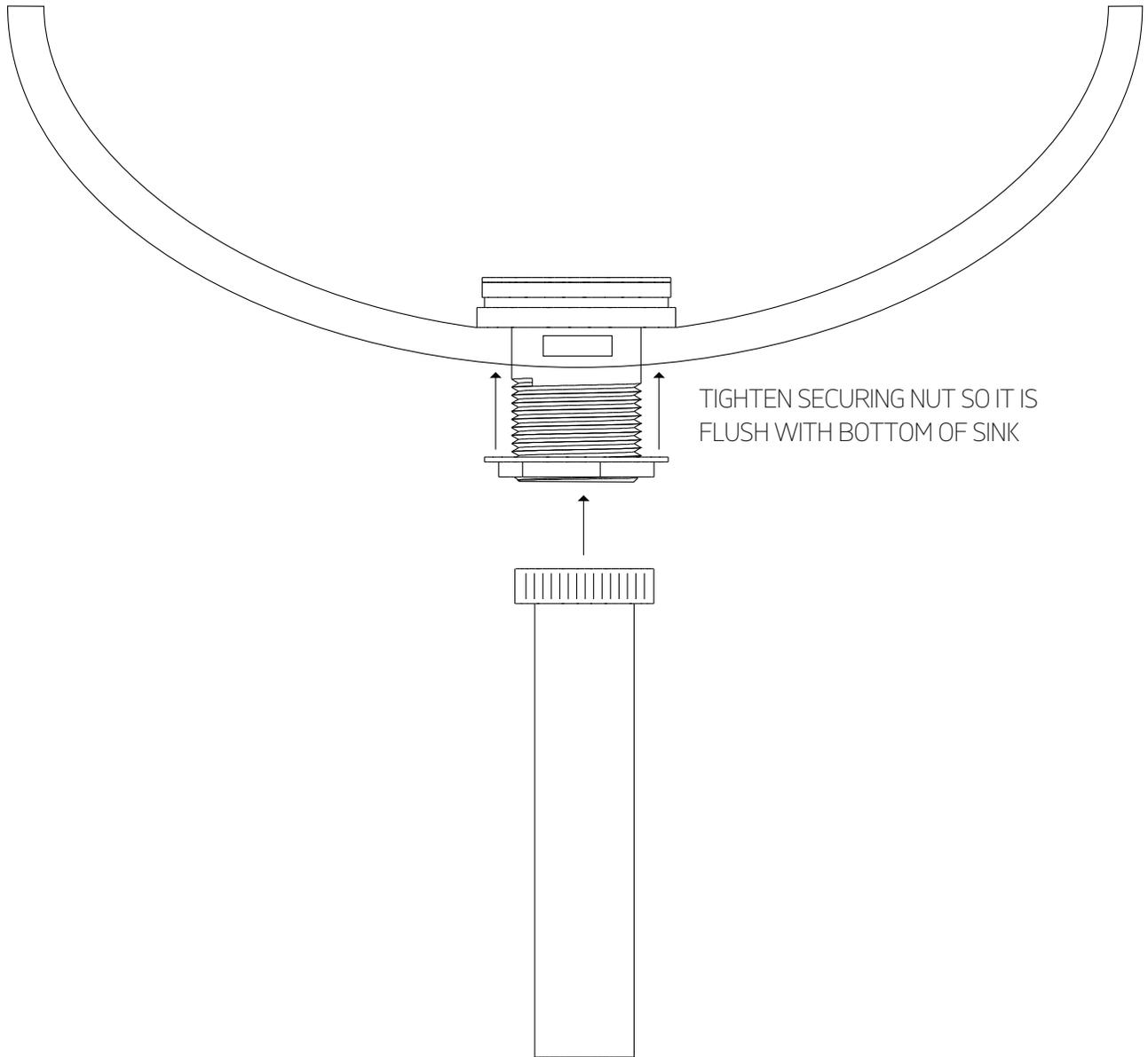
TIGHTEN SECURING NUT SO IT IS
