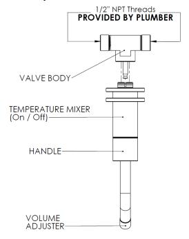
4. Tighten the mixer to the valve body with the allen set screw
