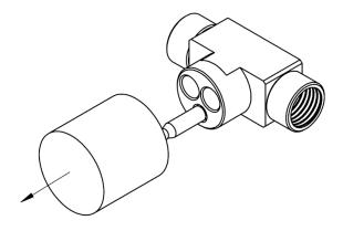
2. Assemble the valve body assuring hot and cold water supply connection.
