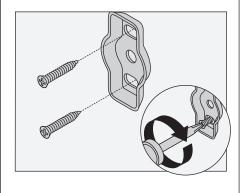
Hang top of accessory on mounting bracket. Lower into position.
