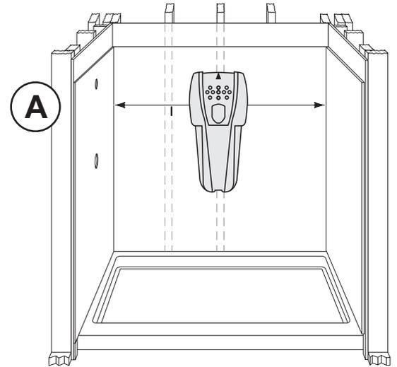
**B.** Mark the location of the studs on the wall panel. A standard height for the recessed shelf would be 42" from the shower floor to the bottom of the opening.
