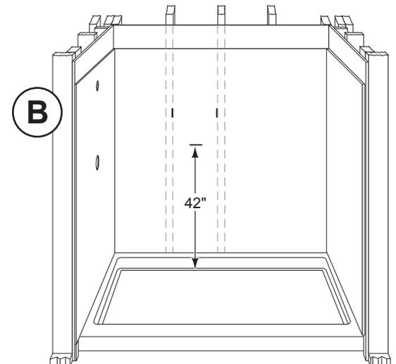
**C. Refer to the images corresponding to your model.** Mark on the panel the measurements shown in the below image. Center the niche between the 2 wall studs as much as possible. Place masking tape over the surface of the panel to protect it against scratching when the hole is cut. Drill a pilot hole through the panel and cementboard. A 3/8" drill bit should be large enough to insert the saber saw blade. Cut the opening for the recessed shelf.
