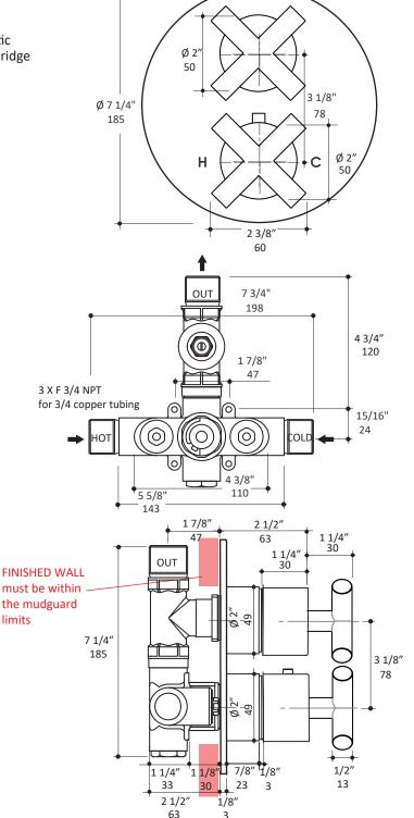
LACAVA reserves the right to revise any dimension or information on this sheet without notice. Dimensions are nominal and may vary within an industry accepted tolerance of 1/4". Drawings provided herein are meant to give the user an idea of the product and are not made to scale. Location of plumbing is meant for reference, your specific applicatuion may vary. Revised: 07/19/2019
