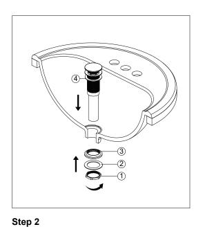
Place the washer (4) underneath the flange of the pop-up body. Slide the pop-up body down through the drain hole on the vessel or basin. From underside, slide the washer (2 & 3) against the bottom of the vessel or basin, thread on the nut (1) and tighten. Do not overtighten.
