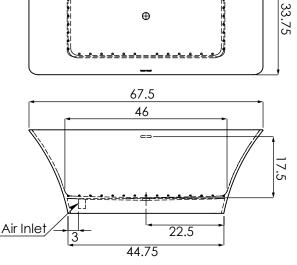
OVERFLOW IS INTEGRAL TO THE TUB
