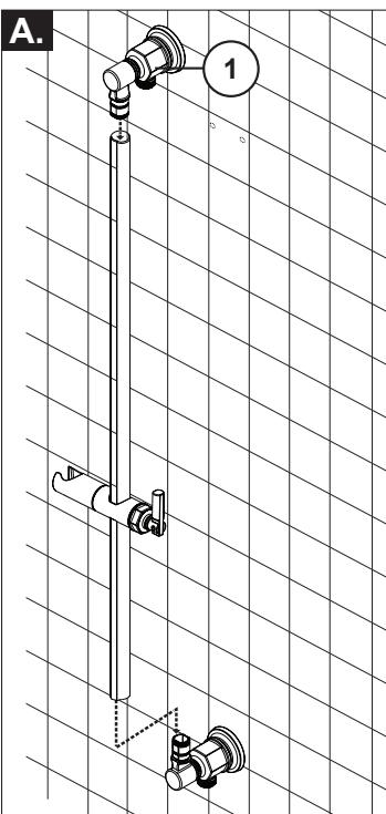
**A. Before drilling holes:** Assemble slide bar by pressing mounting bases fully into bar and ensure that the reference marks are in alignment with upper base plate (1). Adjust marks if necessary.
