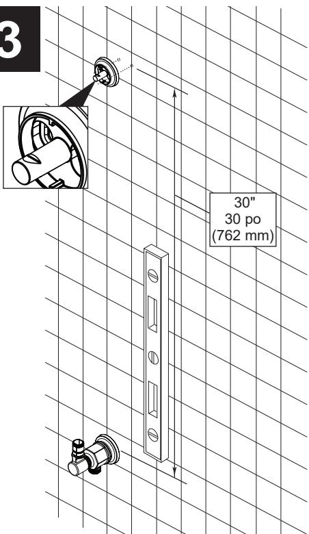
Mark the placement of the upper mounting base plate holes using a level in a vertical line from the lower mounting base. Use upper mounting base plate (1) as a guide. Vertical distance is 30" (762 mm) between bases.
