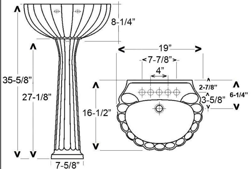
Dimensions of fixture are nominal and may vary within the range of tolerances established by ASME Standard A112.19.2-2018. Dimensions and specifications subject to change without notice.
