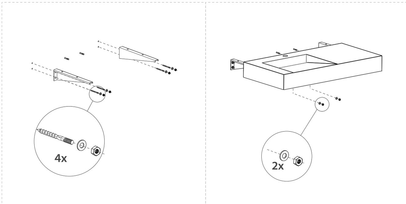
Screw the basin onto the wall brackets. /
