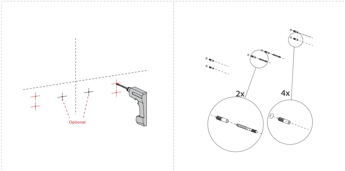
Attach to wall brackets to the wall. /
